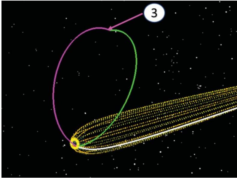
**Figure 2: Phasing orbit plane change & insertion onto interplanetary trajectory (reproduced from [1])**
