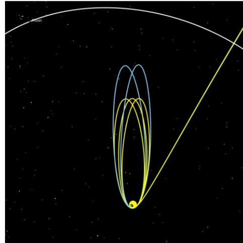
**Figure 4. Two-loop (blue) and a Three-Loop (yellow) phasing orbits shown in Earth-Sun Rotating Coordinates**
