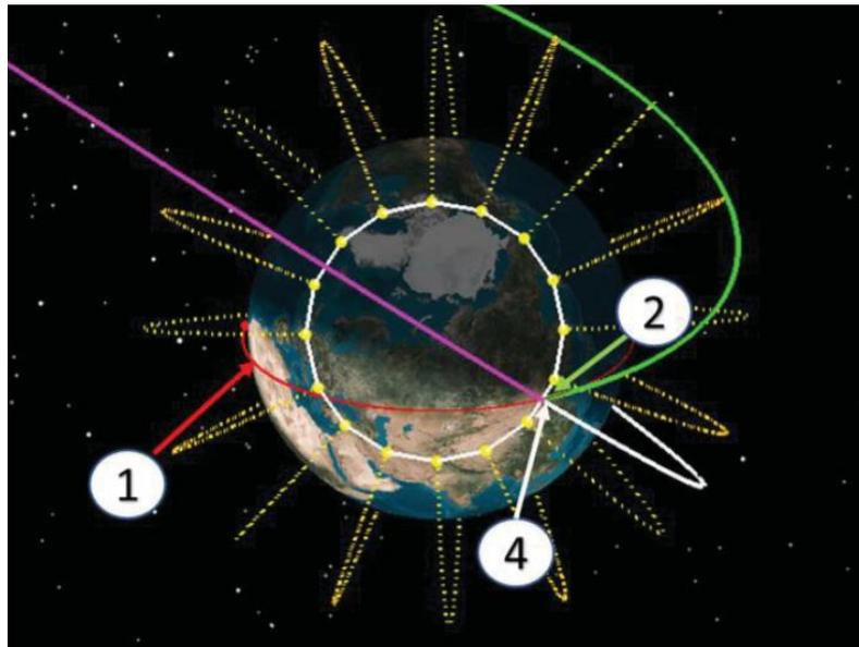
**Figure 1: Initial depot orbit & the locus of injection points (reproduced from [1])**
