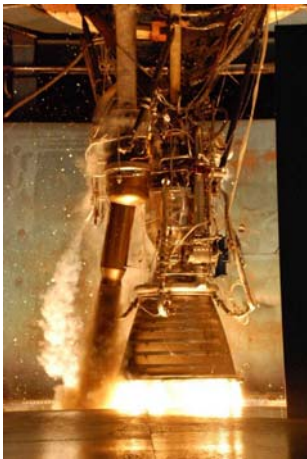
Figure 2. Merlin engine during test fire.
